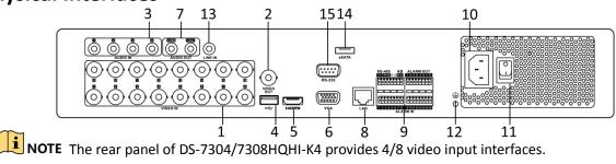
Index Description Index Description RS-485 Serial Interface, Keyboard Interface, 1 VIDEO IN 9 ALARM IN and ALARM OUT 2 **VIDEO OUT** 10 100 to 240 VAC Power Input 3 AUDIO IN, RCA Connector 11 **Power Switch** 4 **USB** Interface 12 **GND** 5 **HDMI** Interface 13 LINE IN 6 VGA Interface 14 eSATA Interface 7 CVBS AUDIO OUT and VGA AUDIO OUT 15 RS-232 Serial Interface
