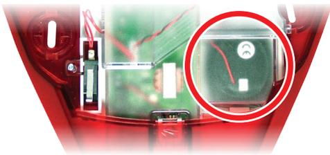
**Engineer hold-off facility.** The Deltabell E's engineer hold-off facility means that when initially powered with the tamper switch open, the sounder will not activate.
